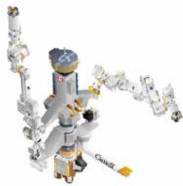
The **Special Purpose Dexterous Manipulator (SPDM)**, known as the “hand,” is an essential tool for maintaining and servicing the Space Station. Its two-handed design allows it to remove and replace
