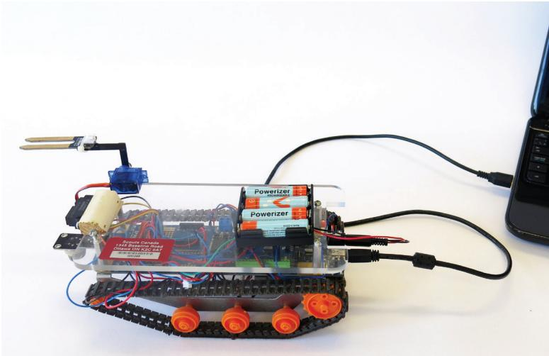
The battery holder is connected through the female barrel connector next to the USB port on the robot. Make sure you charge all the batteries before the meeting.
