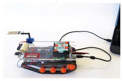
The battery holder is connected through the female barrel connector next to the USB port on the robot. Make sure you charge all the batteries before the meeting.
